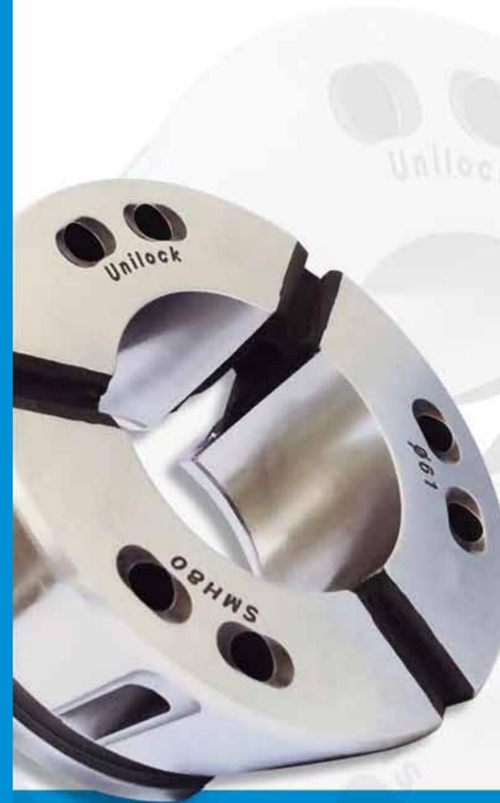
The **UNILOCK SMH COLLETS** are made up from metal inserts, units of vulcanised rubber. This allows the collet to close radially in a perfect manner, blocking the piece along the entire length of the hole and eliminates the intrusion of shavings to pass inside the spindle. Applied to the lathe main spindle it is suitable for bar machining.
